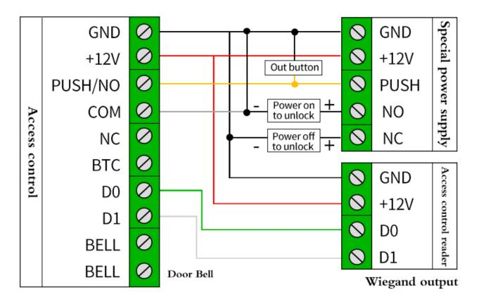
(2) Wiring diagram of ordinary power supply
