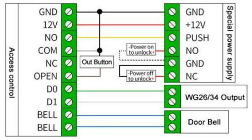
2. Wiring diagram of ordinary power supply
